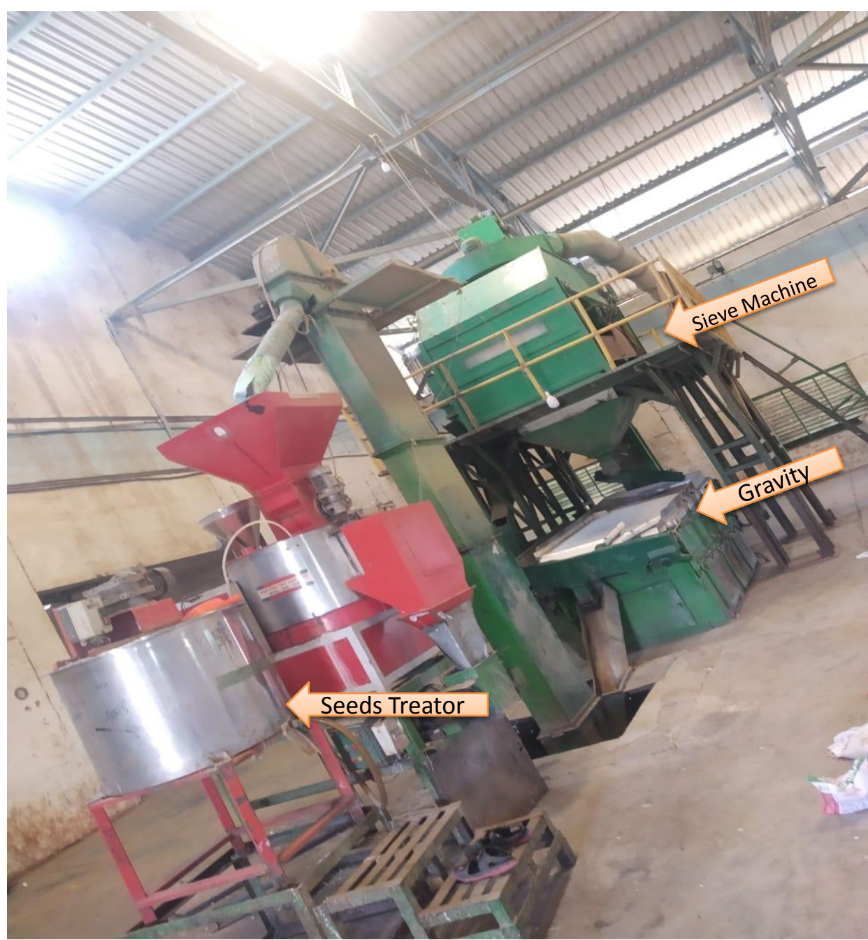
Seed Processing Plant
